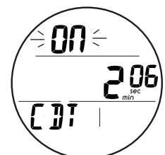
Fig. 137 - CDT STATUS (On, running)
